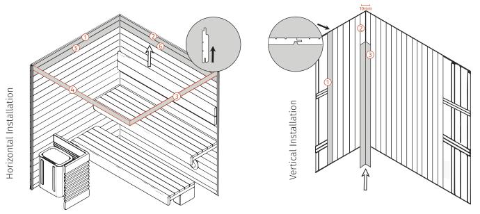
The wall panel is attached to the batten from the groove side using a staple for both vertical and horizontal installation methods. The staple or nail gun should be adjusted to ensure that the staples or nails are driven to the correct depth.
